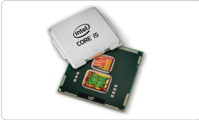
Modern integrated graphics are typically built into the CPU.
